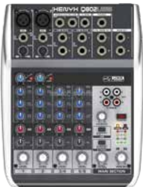
Mixing console for controlling the system
