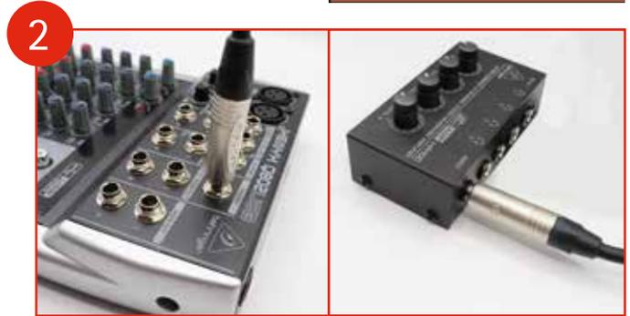
2 Connecting the headphone amplifier to the mixer: Plug the 6.35 mm to 6.35 mm stereo cable into the 'Phones' jack on the mixer and the 'Input' jack on the headphone amplifier.
