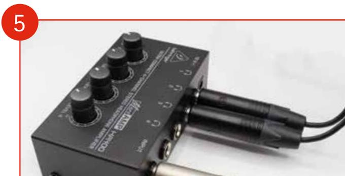
5 Connecting headsets to the headphone amplifier: Plug in 2x headsets with 6.35 mm jack plugs into the headphone amplifier at '1' and '2'.
