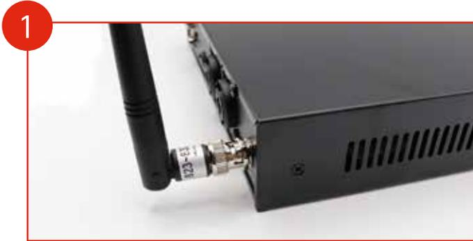
1 Connect the antenna with the bayonet mount to the stationary transmitter.
