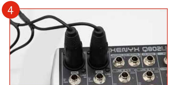
4 Connecting headsets to the mixer: Plug in 2x headsets with XLR connectors into 'MIC 1' and 'MIC 2' on the mixer.
