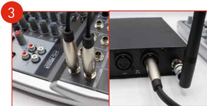
3 Connecting the stationary transmitter to the mixer:
